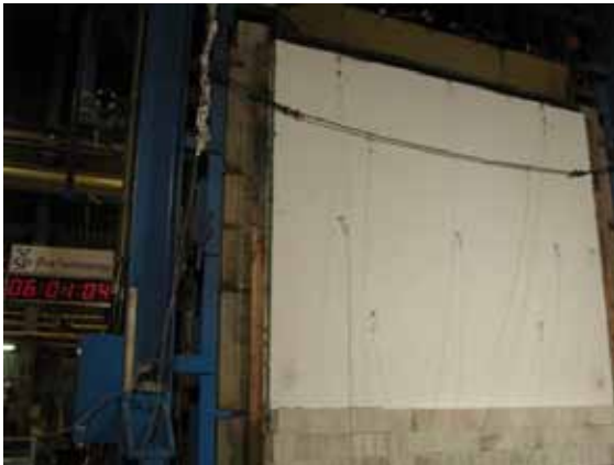
Figure 21 – Fire tests on LE, showing 6 hour fire resistance.
